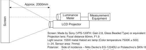
Polarizer: Side of incidence - Nitto Denko's EG-1224DU or Polatechno's SKN-1824ZT or equivalent Side of output light - Polatechno's SHC-128 or equivalent
